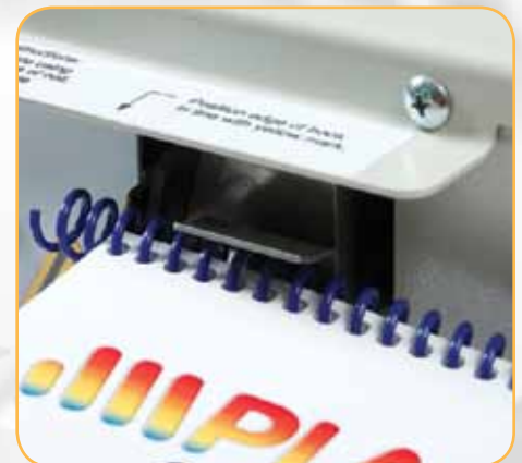
Gateway's TCB crimp technology – Simple dial adjustment to set up that offers consistent coil crimping.
