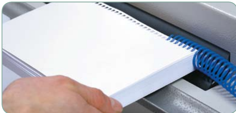
Rollers spin continuously allowing for free use of the operator's hands.
