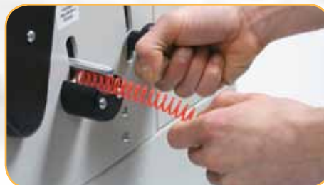
Innovative coil diameter adjustment provides for proper carriage positioning.
