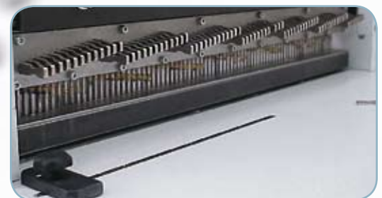
Individually selectable QSA disengagement pins down the full length of the punch die, means extremely fast setup when changing to a different size format.
